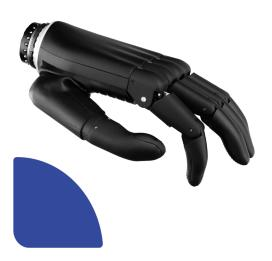
The index finger is active and in a pointing position with the rest of the fingers open. This can be used for working on computer keyboard, typing.
