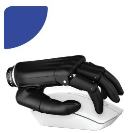
This grip is used to operate a computer mouse. The hand assumes the position of the mouse. The index finger and the middle finger can be controlled to push left and right buttons respectively.
