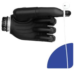
In this grip, the thumb moves to a mid-point and stops. The index finger can be controlled proportionally to form a pinch. Middle, ring and little fingers close fully. This grip can be used for picking up small objects from a table.
