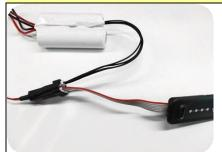
1. Connect **AET-CHR** charging port and **AET-BAT** battery pack to **AET-CON** board via the 7-pin and 4-pin connectors respectively.
