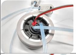
3.Attach the electrodes to the coaxial plug into the EMG/signal input connectors
