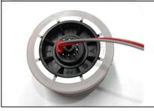
2. Connect **AET-CON** using output 2-pin kidney style connector to the coaxial plug, to the power supply input. Make sure it is properly aligned.
